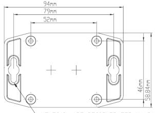
HOLES(2) ARE DESIGNED FOR M4 PAN HEAD MACHINE SCREWS USE.
